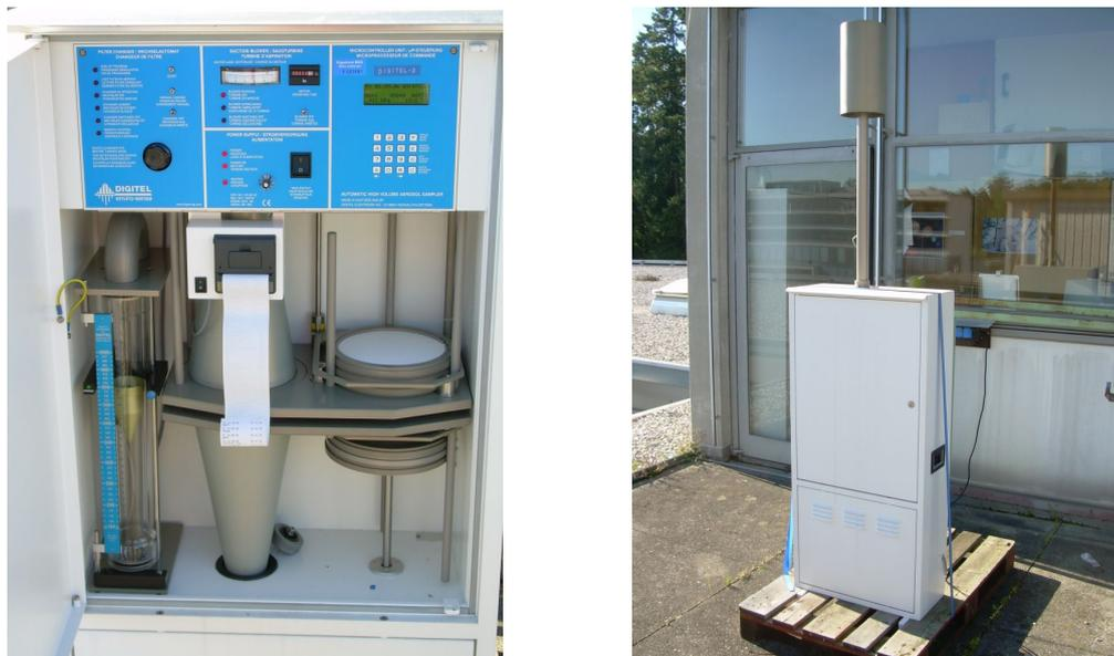
Figure 6.1: The Digital DHA-80 in Fribourg. Inside top on the left the keyboard, below the filter reservoir and on the lower left the floating element
