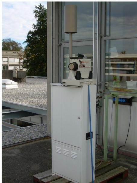
a lead shielding should be provided to the Detective to reduce background and cosmic radiation. These arrangements would require important modifications of the sampler. Moreover the Detective must be modified; a solution has to be found especially for the on-line energy calibration. The first aim of this Master Thesis was to study the feasibility of such a combination, in order to suggest it to the manufacturer of the Digitel sampler.
